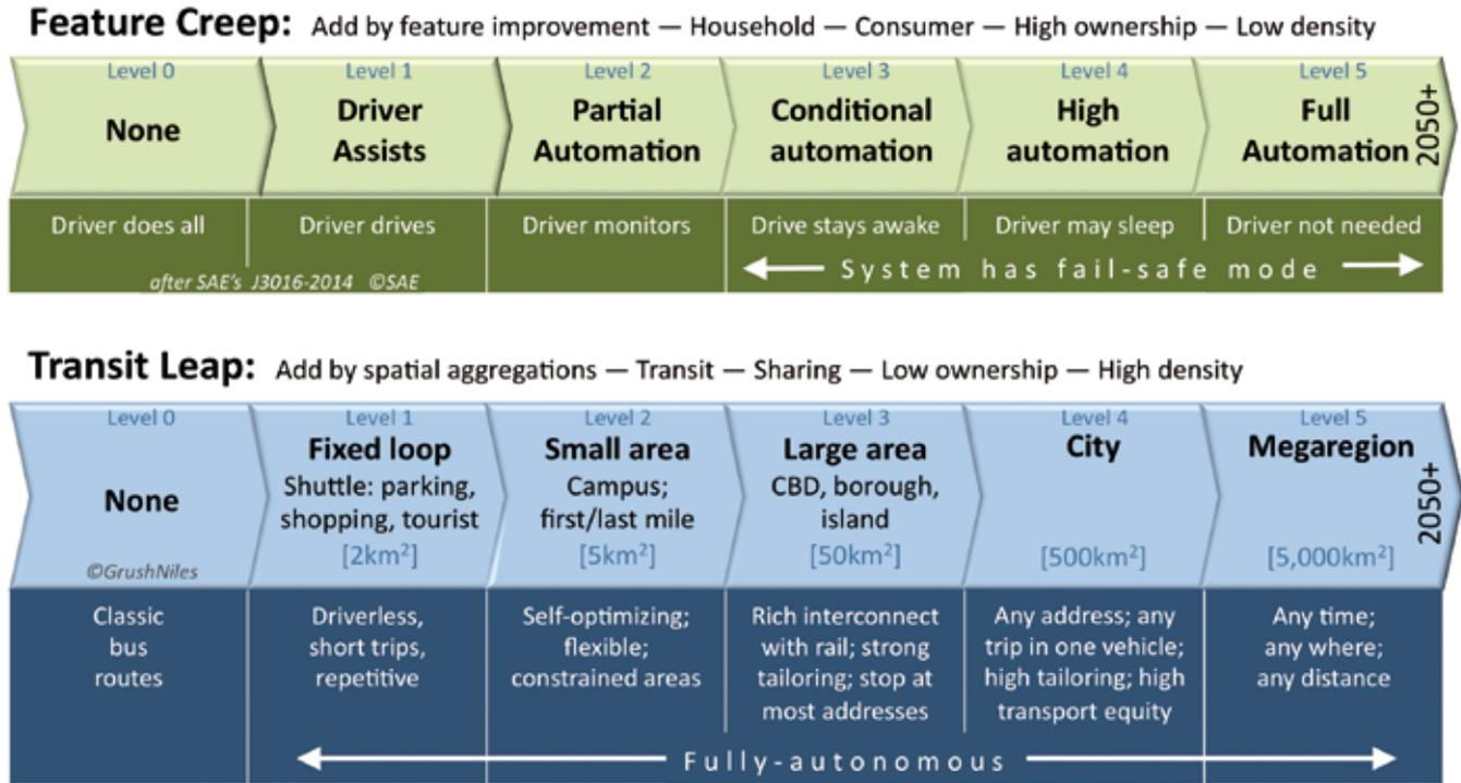
▲ **Figure 2:** [top] Feature Creep as expressed in the five-level autonomous vehicle standard, J3016 from the Society of Automotive Engineers. Only the level 5 vehicle is fully autonomous (no driver controls needed); [bottom] five levels of Transit Leap spreading autonomy by spatial transit extensions rather than by household consumer purchase. All vehicles in Transit Leap Levels 1 through 5 can be fully autonomous SAE Level 5 vehicles
